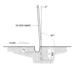
NOTE: ALL DIMENSIONS AND LOCATIONS NOT INDICATED FOR ITEMS APPEARING ON THIS SHEET OR ON THE PLANS SHALL BE AS DIRECTED BY THE ENGINEER. STAKES AND ATTACHMENT OF FILTER FABRIC SHALL BE AS DIRECTED BY THE ENGINEER.
